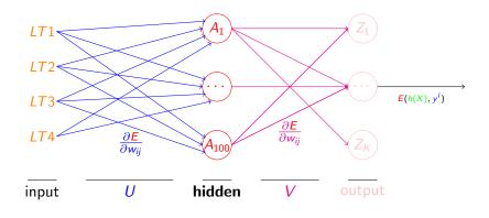
$\frac{\partial E}{\partial w_{ij}} = \sum_{k} \delta_k w_{jk} \sigma'(Z_i) x_i$  $\delta_k \text{ is error of preceding unit.}$
