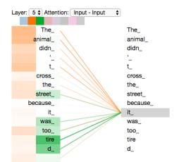
One attention head is focusing most on "the animal", while another is focusing on "tired" http://jalammar.github.io/illustrated-transformer/
